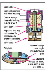
Sectional view of the EVP proportional valve: By press fitting the core closer to the armature, Clippard has increased the magnetic field to create more pull on the armature. The result is a tolerance of  $\pm 10\%$  of maximum flow or better.
