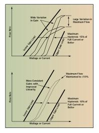
Above: Two typical valve performance curves of a competitor's valve. To compensate for the extreme variations of valve gains, the specification window has been made quite large. Since the gains from valve to valve vary, so does the maximum flow of the valve. Below: A typical Clippard proportional valve hysteresis curve. A relatively consistent linear gain over the entire flow range is much better than the typical "S" shaped gain offered in the market now.
